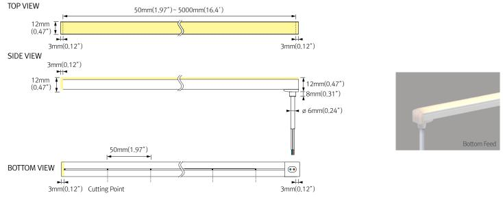
FLXible Neon can be cut every 50mm (1.97"). Please follow the cutting point mark to cut precisely as needed.
